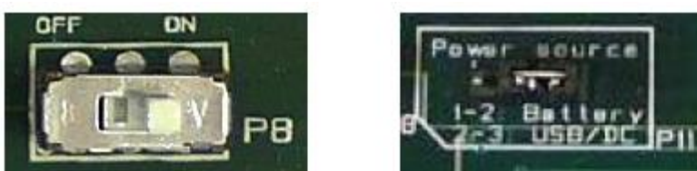
Figure 6: Power Switch and Power Source Selection
